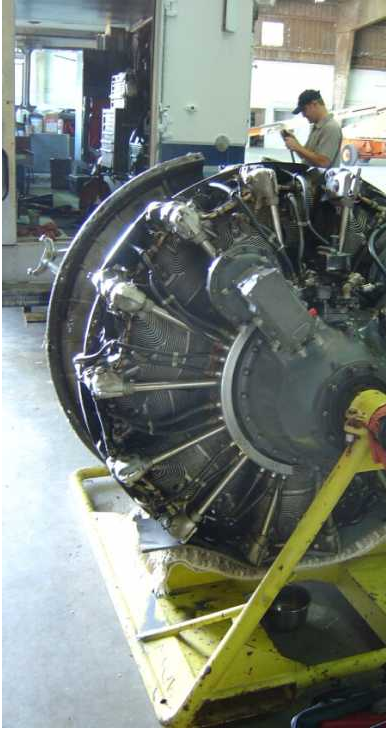
P&W Engine Overhaul
