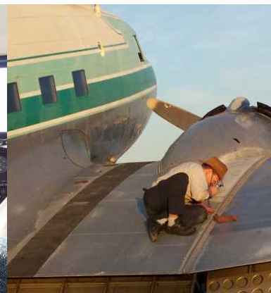
Wing Bolt Inspection
